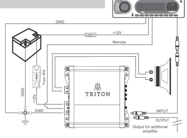
To avoid unwanted noise in the system, join the ground points of the equipment and audio output to only one point.
